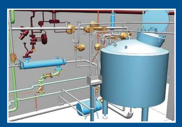
The design of POUs (Points-Of-Use) can be difficult due to several constraints and regulations. As the materials and components used in clean utility systems are often very expensive, it is advisable to complete a thorough design before proceeding to building. 3D design of a POU/ sample point on a WFI system (above) and the completed POU (right).
