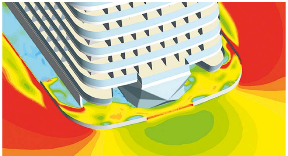
▲ Figure 4. An example of a CFD simulation for a full scale wind tunnel test on a cruise ship to detect the comfort level in the superstructures and outer decks.
