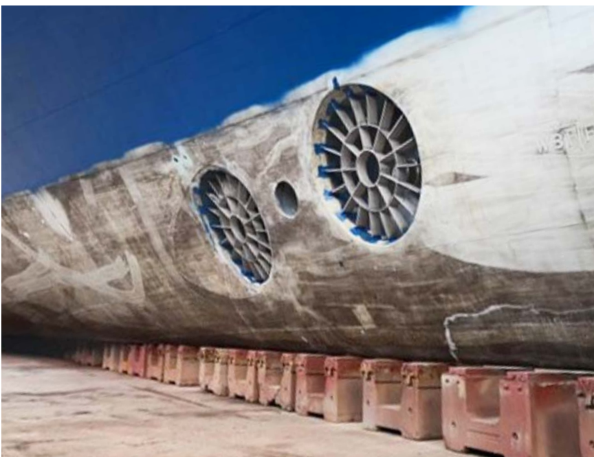
Figure 7: Elogrids installed on Gabriella bow thruster tunnels.
